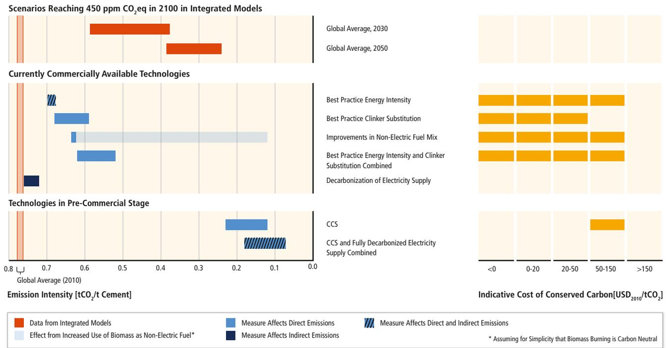
**Figure 10.7** | Indicative CO<sub>2</sub> emission intensities and levelized cost of conserved carbon in cement production for various production practices/technologies and in 450 ppm scenarios of selected models (AIM, DNE21+, IEA ETP 2DS) (for data and methodology, see Annex III).
