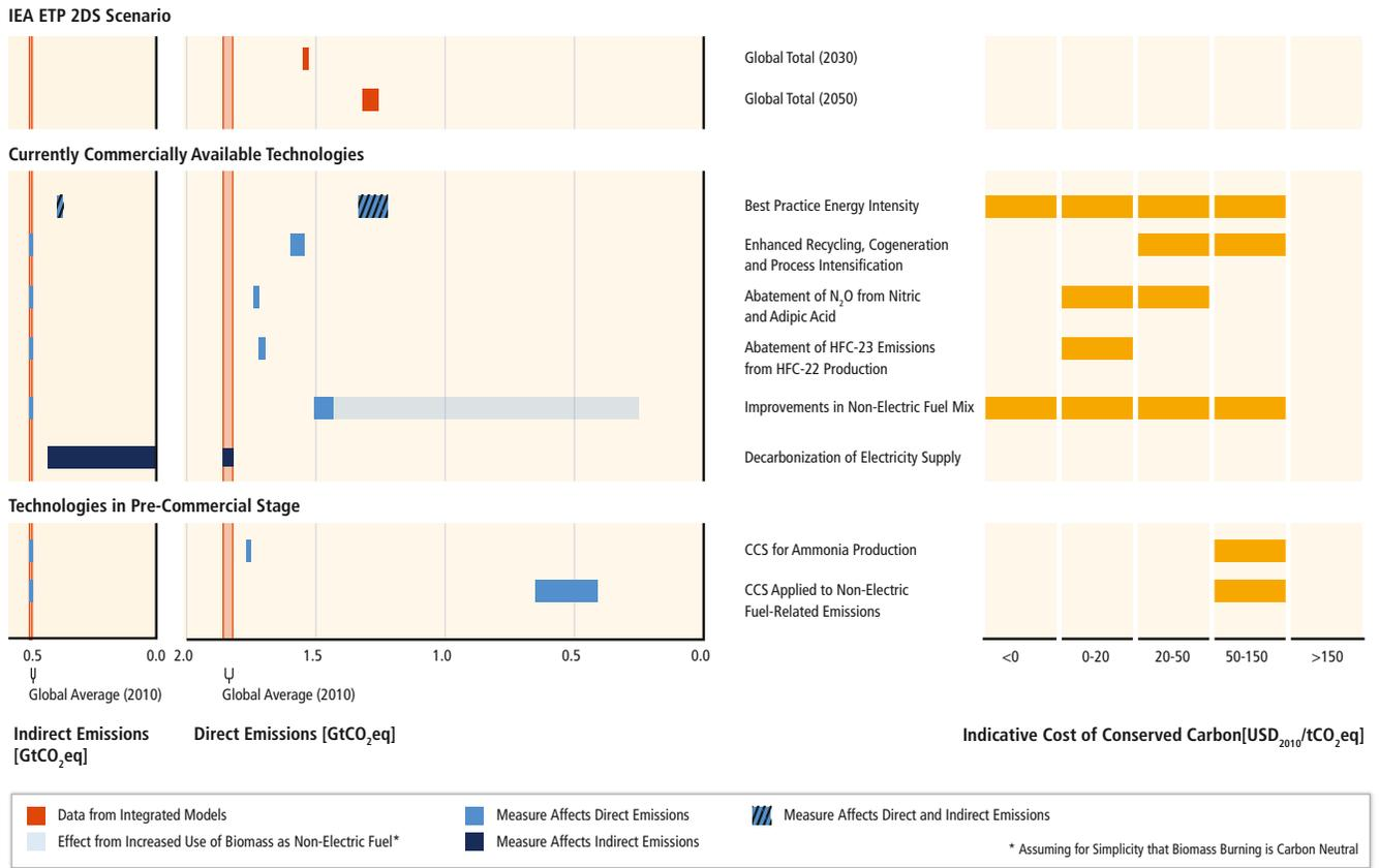
**Figure 10.9** | Indicative global indirect (left) and direct (right) CO<sub>2</sub>eq emissions and leveled cost of conserved carbon resulting from chemicals production for various production practices/technologies and CO<sub>2</sub> emissions in IEA ETP 2DS scenario (for data and methodology, see Annex III).
