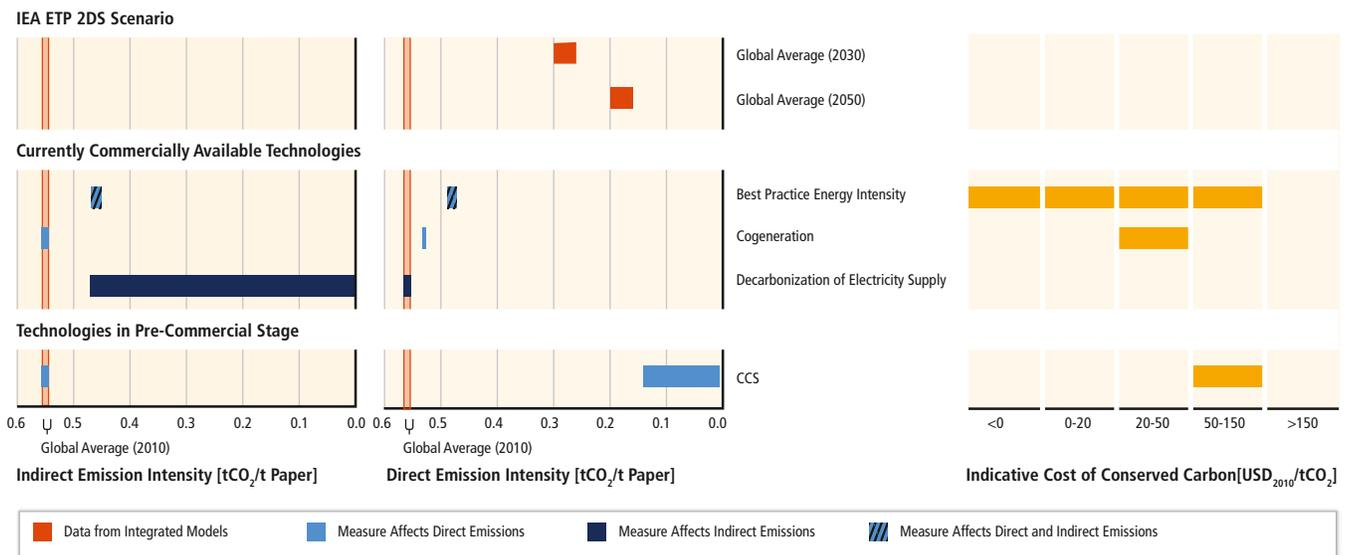
**Figure 10.10** | Indicative global indirect (left) and direct (right) CO<sub>2</sub> emission intensities and leveled cost of conserved carbon in paper production for various production practices/technologies and in IEA ETP 2DS scenario (for data and methodology, see Annex III).
