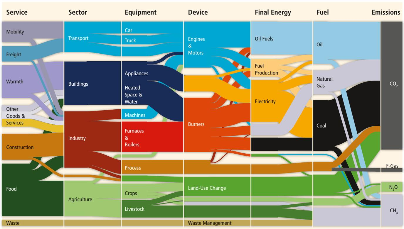
**Figure 10.1** | A Sankey diagram showing the system boundaries of the industry sector and demonstrating how global anthropogenic emissions in 2010 arose from the chain of technologies and systems required to deliver final services triggered by human demand. The width of each line is proportional to GHG emissions released, and the sum of these widths along any vertical slice through the diagram is the same, representing all emissions in 2010 (Bajželj et al., 2013).
