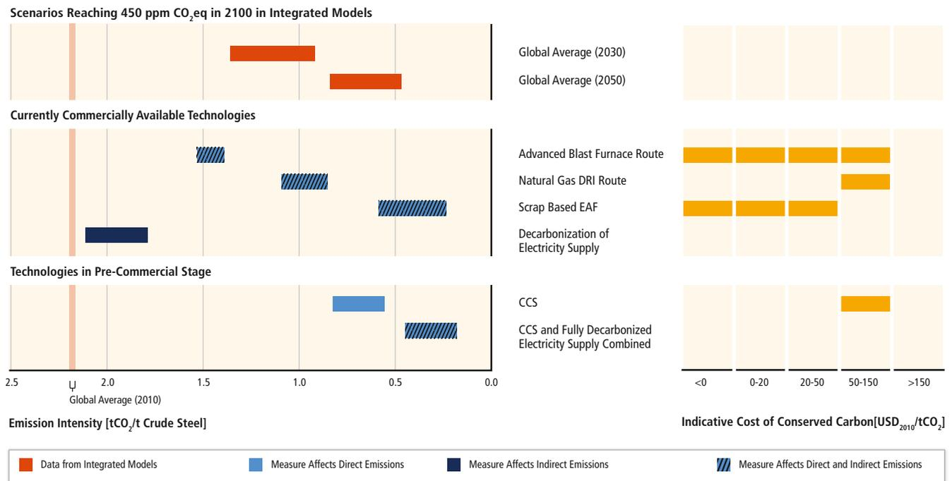
**Figure 10.8** | Indicative CO<sub>2</sub> emission intensities and levelized cost of conserved carbon in steel production for various production practices/technologies and in 450 ppm scenarios of selected models (AIM, DNE21+, and IEA ETP 2DS) (for data and methodology, see Annex III).
