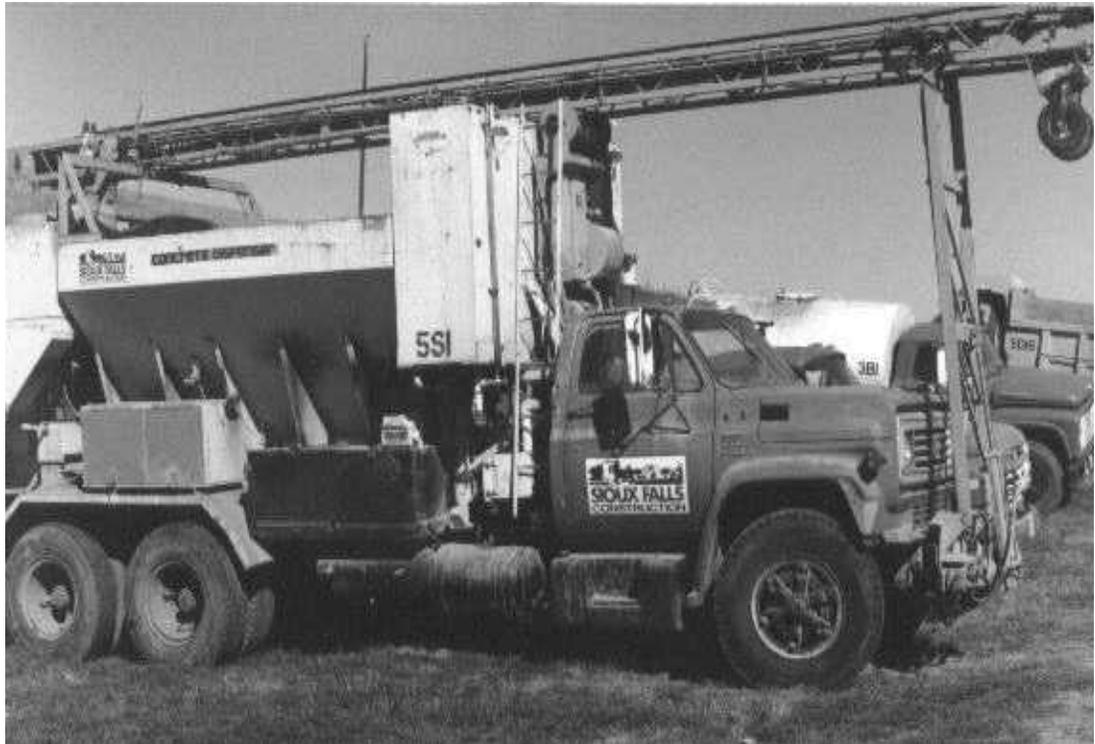
An annual calibration and inspection by the SDDOT will be required for each mixer before the start of the first project each year. The calibration establishes the meter count, i.e., the number of revolutions, and discharge time in seconds required to dispense 94 pounds of cement. Gate openings and pointer adjustments for aggregates and general operating condition of the equipment will also be inspected, as per the manufacturer's recommendations.
