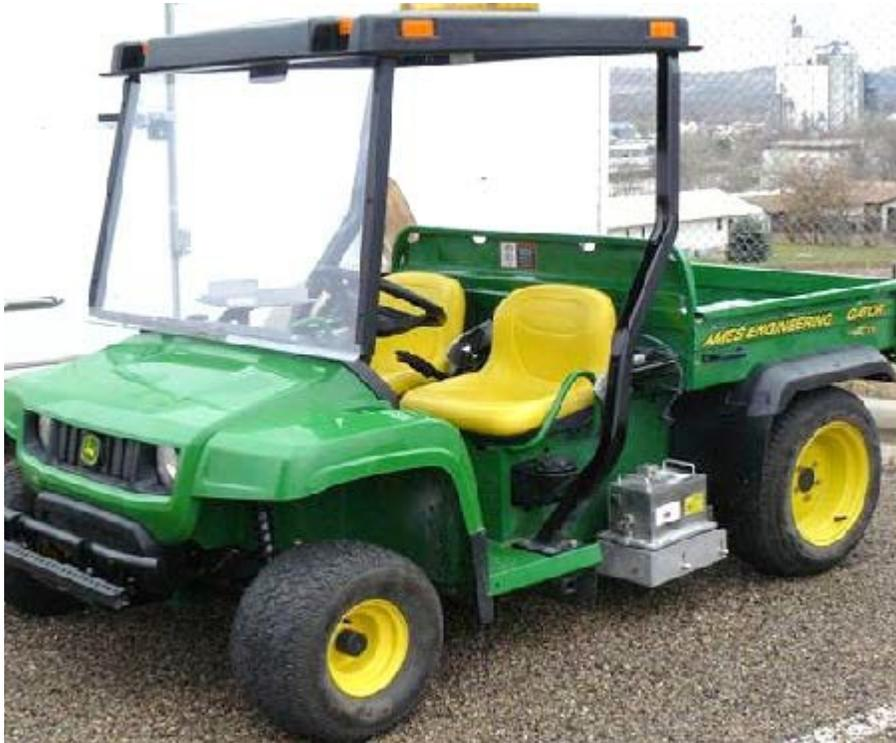
**Figure 8.13** High Speed Profiler
