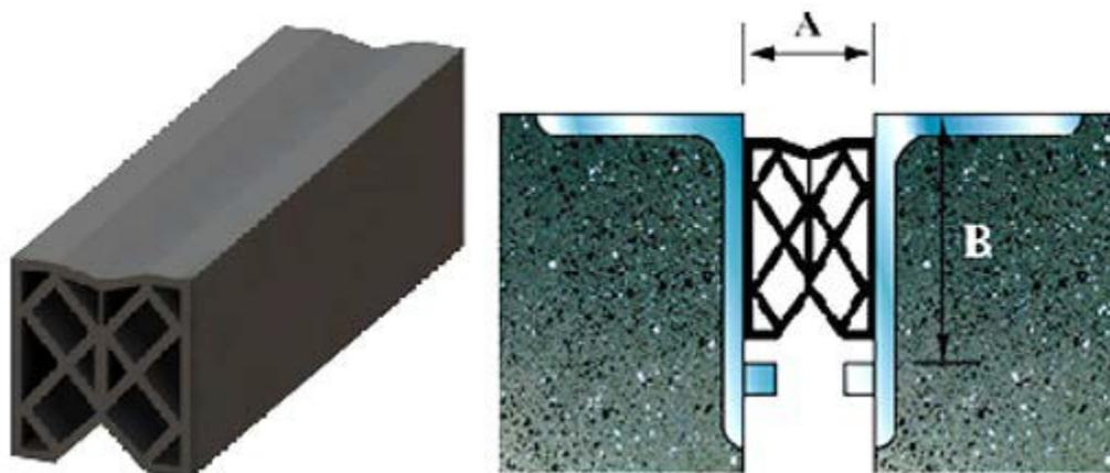
**Figure 7.15** Compression Seal Joint installed.
