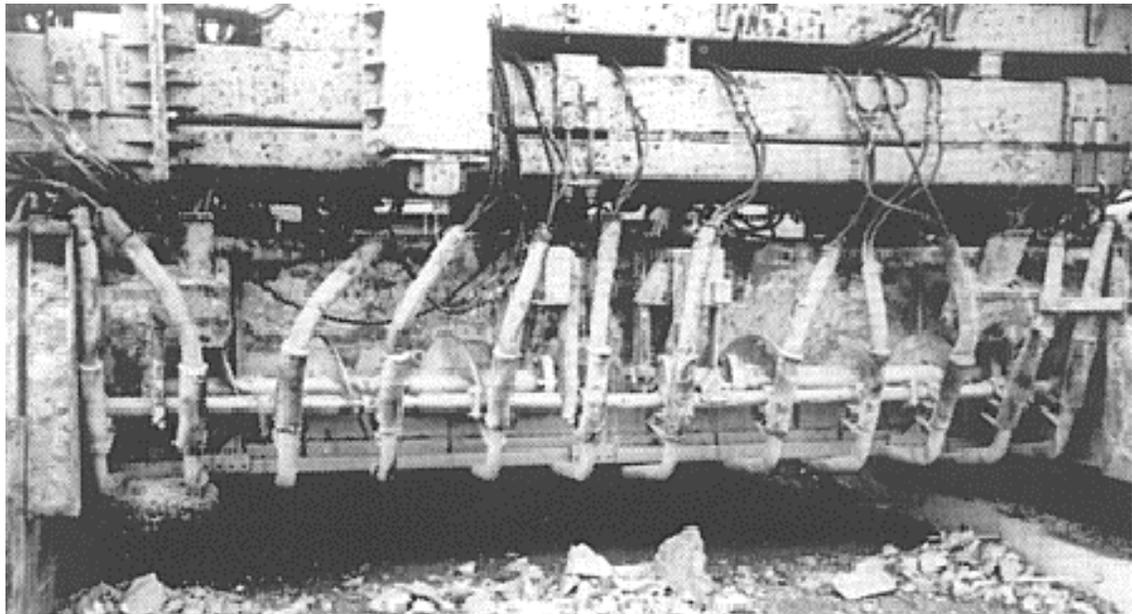
**Figure 5.19** Internal tube vibrators areas of influence.
