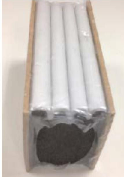
**Figure 7.18** Bituminous Mix Expansion Joint
