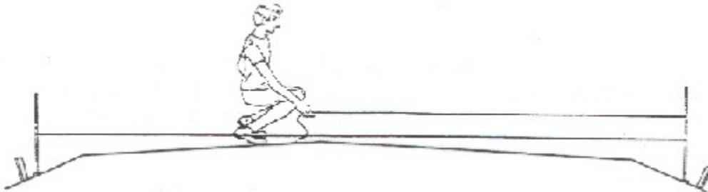
Find the roadway centerline by measuring the offset distance from one of the hubs (Figure 2.25).
