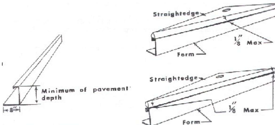
**Figure 3.2** Form specifications, plan view.
