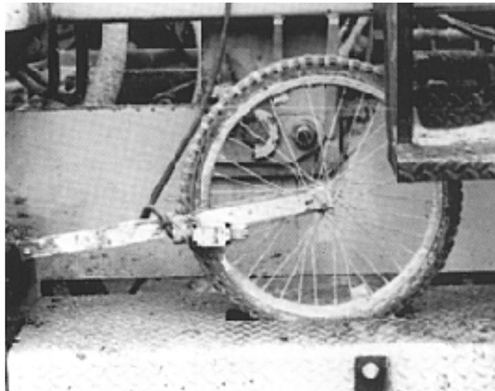
An inserter unit mounted on the side of a slipform paver consists of a measuring device and a tie bar inserter to place the steel. Sometimes the measuring device is a small wheel that rides on one track of the paver (Figure 3.18). The wheel measures the forward movement of the paver and at the predetermined intervals an electronic impulse is sent to the placement unit. For a side
