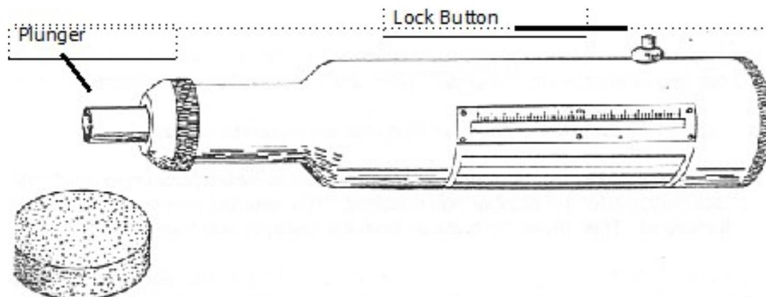
When placing the hammer in the case, put the plunger against something solid and push it all the way in. Then press the lock button on the side. There is, also, a scale marked 0 to 100 on the side of the Swiss Hammer. In the center of this scale is a small rider with a line in the center.
