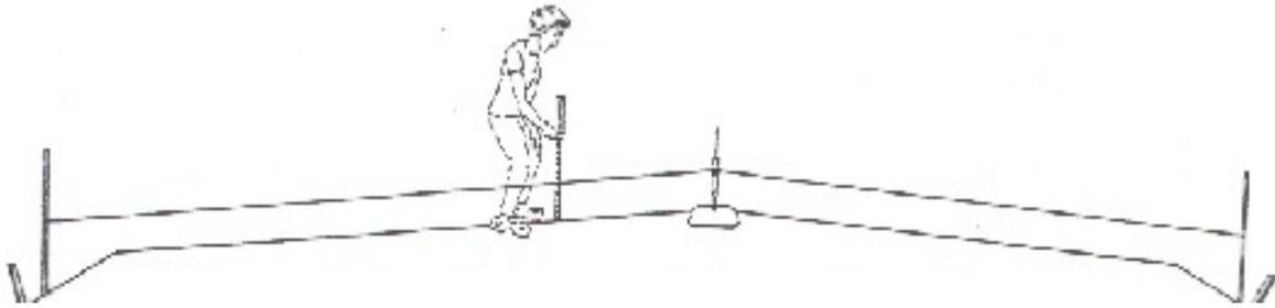
Use a ruler to measure the distance (Figure 2.27) between the string-line and finegrade at intervals along the stringline from one intended pavement edge to the other side. Document the results of the check in the diary.
