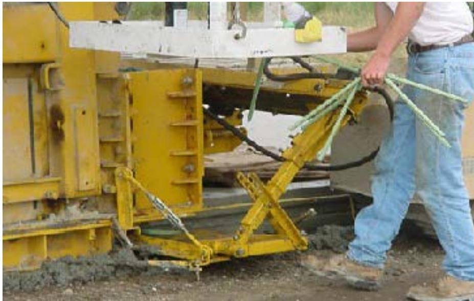
**Figure 3.20** Centerline tie bar inserter (not allowed).
