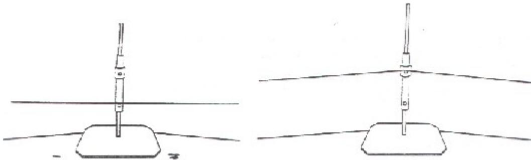
Adjust the sleeve of the crown checker so the bottom arm just touches the stringline. Put the stringline on the top arm (Figure 2.26). The string is now at the elevation and has the same slope as the top of the pavement.
