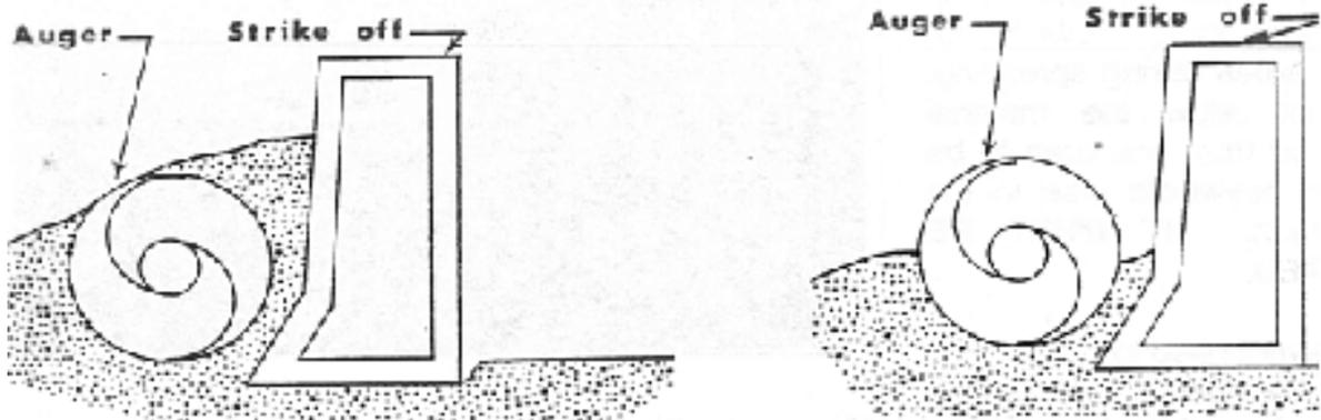
Care should be exercised to maintain a constant and continuous movement of the paver. Any starts and stops of the paver can cause the machine to ride up over the mix and result in bumps in the pavement and a poor riding surface. The forward speed of the paver should be as uniform as possible but should be varied according to the speed of concrete placement.
