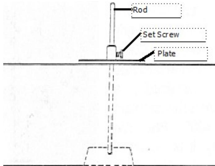
**Figure 5.28** Depth check in progress.
