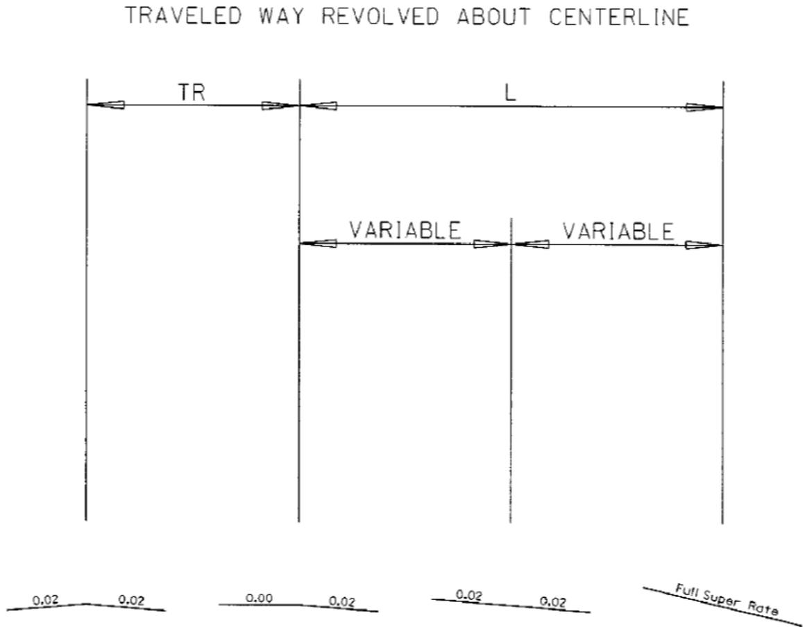
**Figure 2.12** Superelevated section, no crown in pavement.
