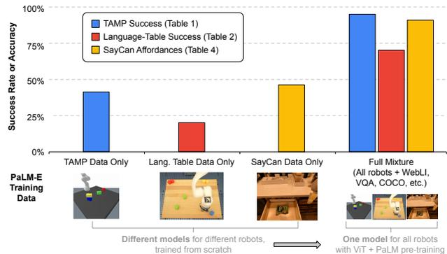
Figure 3: Overview of *transfer* learning demonstrated by PaLM-E: across three different robotics domains, using PaLM and ViT pretraining together with the full mixture of robotics and general visual-language data provides a significant performance increase compared to only training on the respective in-domain data. See Tab. 1, Fig. 4, Tab. 2, Tab. 4 for additional data in each domain.
