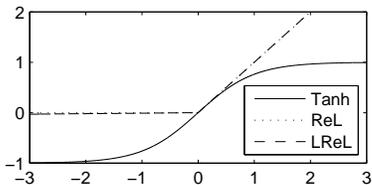
Figure 1. Nonlinearity functions used in neural network hidden layers. The hyperbolic tangent (tanh) function is a typical choice while some recent work has shown improved performance with rectified linear (ReL) functions. The leaky rectified linear function (LReLU) has a non-zero gradient over its entire domain, unlike the standard ReL function.
